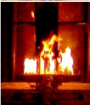
Henikwon Busduct System under ASTA Type Test
