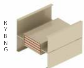
3-phase, 4-wire with Internal ground & 50% or 100% Neutral
