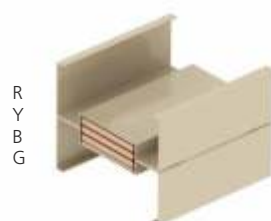
3-phase 3-wire with Internal ground
