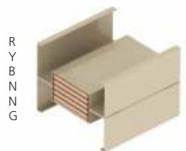
3-phase, 5-wire with Internal ground & 200% Neutral
