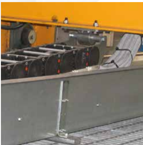
Program LF58: Installed in sliding configuration in an automatic warehouse
