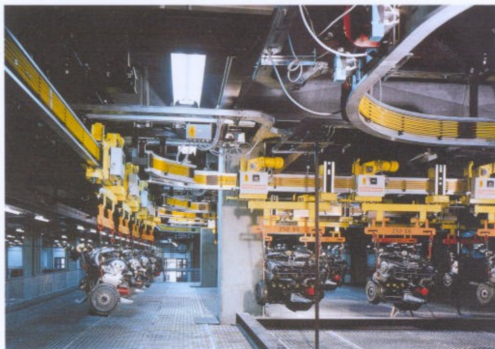
Back-up line installation of an electrically driven trolley conveyor for the transport of motors.
