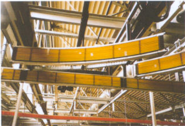
10-pole electrically driven switch for a trolley conveyor with variable feed points.
