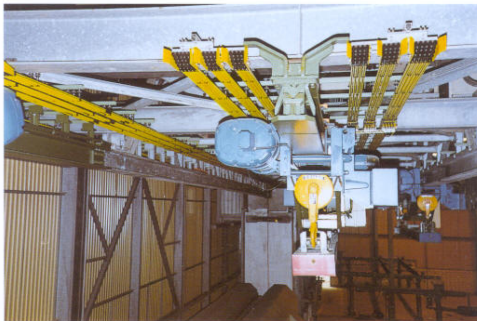
Automatic crane installation for transfer operation with pick up guides in a zinc coating plant.
